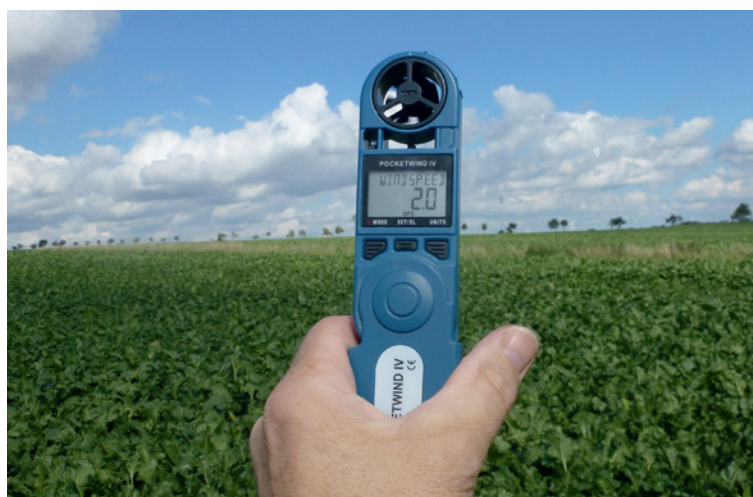
Figure 13: Use a wind velocity meter to determine the current wind speed (© Garrelts)
