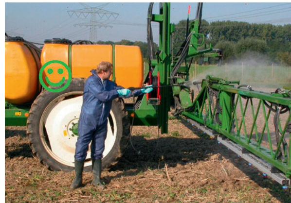
Figures 11 to 12: Correct rinsing procedures prevent point pollution.
