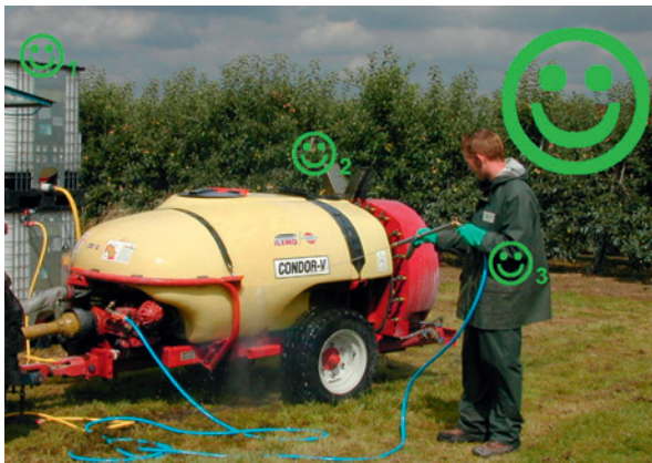
Figures 11 to 12: Correct rinsing procedures prevent point pollution.
