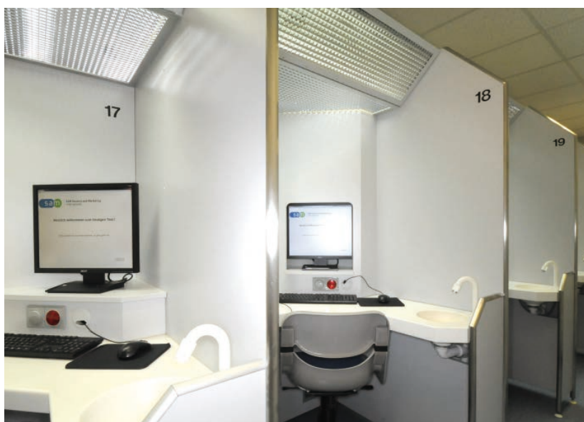
Figure 5: Test cabins for sensory tests
