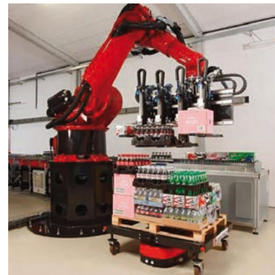
Picture 8: Automatic creation of a mixed pallet in a driverless transport system. Product defines the packing schematic, robot programme adapts, autonomous vehicle delivers the shipping pallet to the loading dock ready for dispatch
